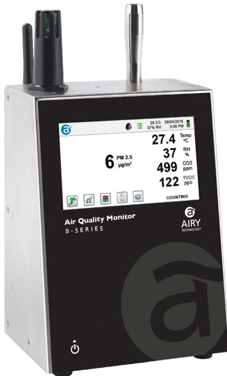
The Airy Technology® B7301-AQM1 and B7301-AQM2 Air Quality Monitors measure particles from 0.3 to 25.0 µm at a flow rate of 0.1 CFM (2.83 LPM). These user-friendly instruments display up to six particle size channels, temperature, relative humidity, and CO<sub>2</sub> (AQM1) or CO<sub>2</sub> + TVOC (AQM2).
