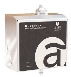
The R2301 and R2501 particle counters provide a range of particle size measurement from 0.3 or 0.5 to 25.0  $\mu$ m at a flow rate of 0.1 CFM (2.83 LPM). These sensors allow for efficient particle counting with specifications that exceed the ISO 21501-4 and JIS B9921 calibration standards.
