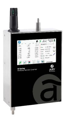
The Airy Technology® R5501-30 Remote Particle Counter measures 0.5 to 75.0 µm and are the most feature advanced remote particle counters available. Integration is easy into a building automation and cleanroom management system via Ethernet, or (optional) Wireless 802.11 b/g, RS485 or RS232. Integrated web server displays instrument screen through any browser.
