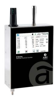
The Airy Technology® R5510 Remote Particle Counter measures 0.5 to 25.0  $\mu m$  and is the most feature advanced remote particle counters available.
