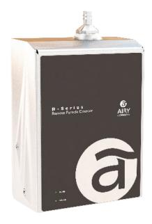
The 9300P IoT particle counter provides a range of particle size measurement from 0.3 to 25.0  $\mu$ m at a flow rate of 1.2 LPM. These sensors allow for efficient particle counting with specifications that exceed the ISO 21501-4 and JIS B9921 calibration standards.
