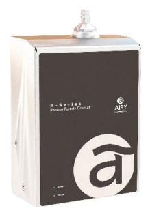
The R9301 and R9501 IoT particle counters provide a range of particle size measurement from 0.3 to 25.0  $\mu$ m at a flow rate of 0.1 CFM (2.83 LPM). These sensors allow for efficient particle counting with specifications that exceed the ISO 21501-4 and JIS B9921 calibration standards.
