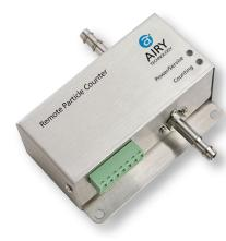
The Airy Technology® P230 Remote Particle Counter measures 0.3 µm and 0.5 µm with a flow rate of 0.1 CFM (2.83 LPM). Integration is easy into a real-time monitoring or building management system via Modbus RTU. The P200 models are the smallest 0.1 CFM remote particle counters on the market and have easy mounting options. The Airy Technology® P230 unit complies with ISO 21501-4 and includes a 1 year limited warranty.
