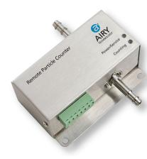
The Airy Technology® P231 Remote Particle Counter measures 0.5 µm and 5.0 µm with a flow rate of 1.0 CFM (28.3 LPM). Integration is easy into a real-time monitoring or building management system via Modbus RTU. The P200 models are the smallest 1.0 CFM remote particle counters on the market and have easy mounting options. The Airy Technology® P231 unit complies with ISO 21501-4 and includes a 1 year limited warranty.
