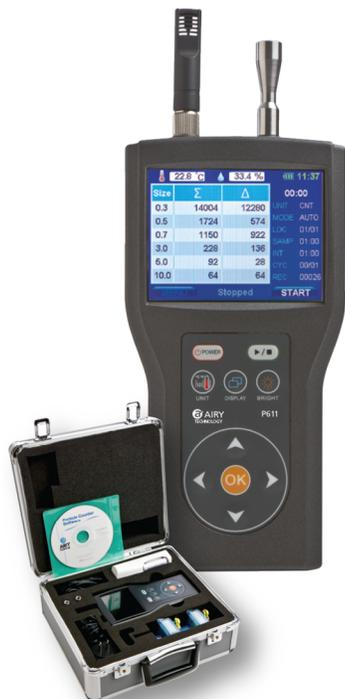
The Airy Technology® P611 handheld particle counter measures 0.3 µm to 10.0 µm with a flow rate of 0.1 CFM (2.83 LPM).
