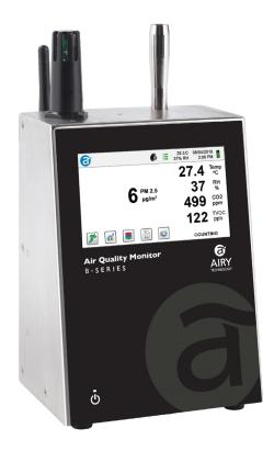
The Airy Technology® B7301-AQM1 and B7301-AQM2 Air Quality Monitors measure particles from 0.3 to 25.0  $\mu$ m at a flow rate of 0.1 CFM (2.83 LPM). These user-friendly instruments display up to six particle size channels, temperature, relative humidity, and CO2 (AQM1) or CO2 + TVOC (AQM2).
