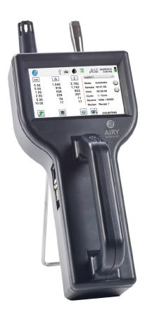
The Airy Technology® H8300 Particle Counters are purpose-built for ambient and indoor air quality monitoring, industrial hygiene, environmental research, and health & safety applications. Featuring a 1.2 LPM flow rate, the 8300 is optimized for high-concentration environments providing improved accuracy, reduced coincidence loss, and extended instrument lifespan in comparison to higher-flow models.
