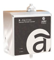
The Airy Technology® R2510 and R2510-2 Remote Particle Counters provide a range of particle size measurement from 0.5 to 25.0 µm at a flow rate of 1.0 CFM (28.3 LPM) and are designed for continuous monitoring in cleanrooms and other controlled environments. With two or four particle size channels, these instruments deliver targeted contamination detection with real-time data collection and configurable alarms for immediate incident reporting and local visual alerts.
