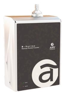
The R301P and R501P particle counters provide a range of particle size measurement from 0.3 to 25.0  $\mu$ m at 0.1 CFM (2.83 LPM) flow. These sensors allow for efficient particle counting with high accuracy and resolution that meet or exceed ISO 21501-4 and JIS B9921 for the calibration of a particle counter.
