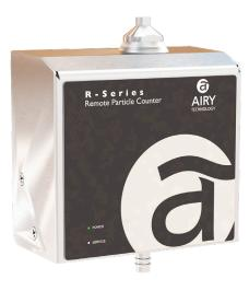
The R510 and R510-2 particle counters provide a range of particle size measurement from 0.5 to 25.0  $\mu$ m at a flow rate of 1.0 CFM (28.3 LPM). These sensors allow for efficient particle counting with specifications that exceed the ISO 21501-4 and JIS B9921 calibration standards.
