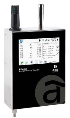
The Airy Technology® R5501-30 Remote Airborne Particle Counter measure particles from 0.5 to 75.0  $\mu$ m at a flow rate of 0.1 CFM (2.83 LPM). These user-friendly instruments display up to six selectable particle size channels, along with optional temperature and relative humidity measurements.
