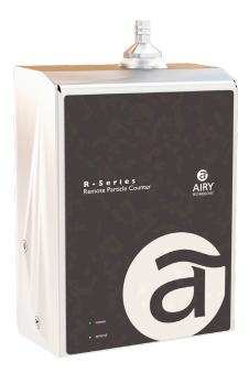
The Airy Technology® R9300P Remote Airborne Particle Counters are designed for continuous monitoring in cleanrooms and other controlled environments. With 30 user-selectable particle size channels ranging from 0.3 up to 25.0  $\mu m$  and a quiet 1.2 LPM internal pump, these instruments deliver targeted contamination detection with real-time data collection and configurable alarms for immediate incident reporting and local visual alerts.
