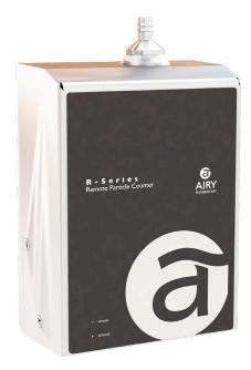
The Airy Technology® R9301P and R9501P Remote Airborne Particle Counters are designed for continuous monitoring in cleanrooms and other controlled environments. With 30 user-selectable particle size channels ranging from 0.3 or 0.5 up to 25.0µm and a quiet 0.1 CFM (2.83 LPM) internal pump, these instruments deliver targeted contamination detection with real-time data collection and configurable alarms for immediate incident reporting and local visual alerts.
