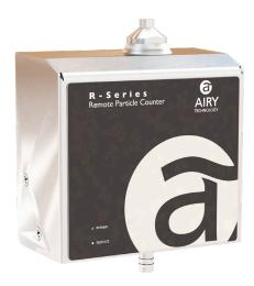
Airy Technology® R9510 Remote Airborne Particle Counters monitor particle sizes ranging from 0.5 to 25  $\mu$ m across six user-selectable channels at a flow rate of 1.0 CFM (28.3 LPM). These instruments are designed for collecting particle data in cleanrooms or other controlled environments, and seamlessly integrate with Particles Plus® Software, facility monitoring systems, or local data collection platforms.
